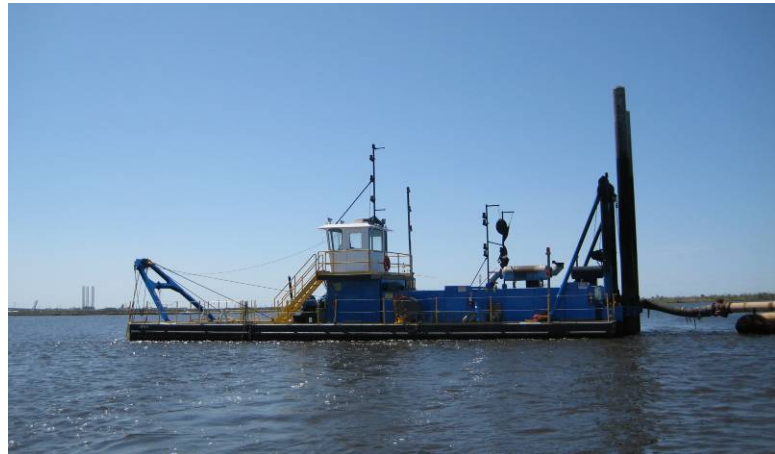
ENCO's Dredge Ruth, an 18"x16" cutter suction dredge, was used to remove sediment and increased the river's depth by 6 feet.
