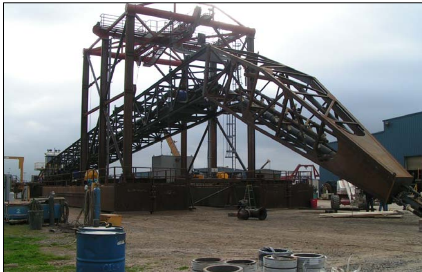
After fabrication and testing, the Marlin mining dredge was disassembled and loaded onto 23 tractor trailers for transport to the Florida "pond" where it will operate until the middle of the 21st century.
